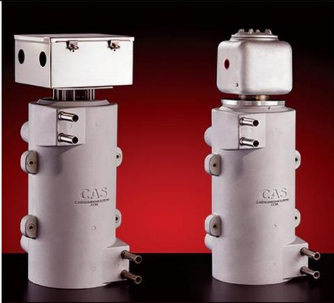
CAST-X 4000 Circulation Heaters from Cast Aluminum Solutions. These units feature dual 1 inch OD (2.5 cm) flow-tubes made of seamless 316L stainless steel. The CAST-X 4000 is capable of heating flammable liquids or gases, even under tremendous operating temperatures.
